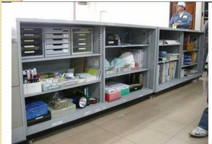
5S – all material identified and in its place. In the furniture, the wheels to facilitate moving.
