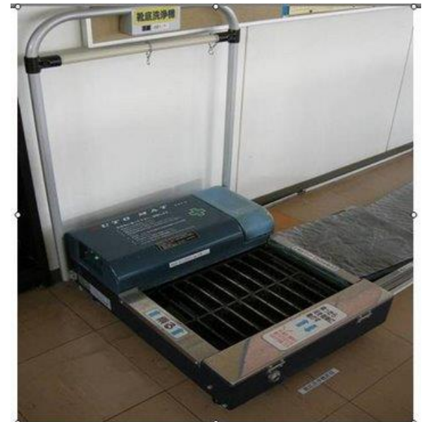
Device to clean foot. Before come in the production hall, everybody must clean the foot
