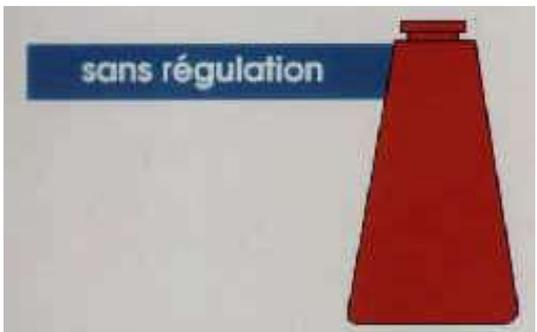
The diagram shows a red extruder die with a blue label 'sans régulation' to its left. The extruded parison is a red cone that is wider at the top and tapers towards the bottom, indicating an irregular thickness.                                               |                            |                 |
