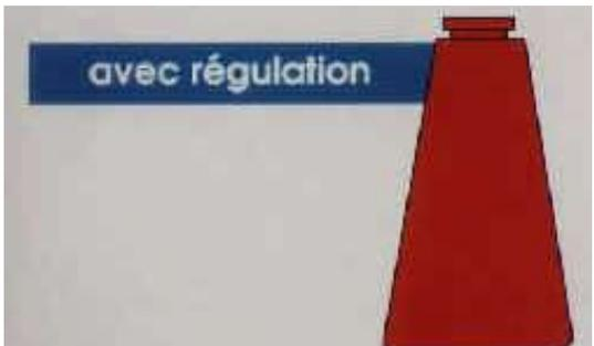
The diagram shows a red extruder die with a blue label 'avec régulation' to its left. The extruded parison is a red cone that is wider at the top and tapers towards the bottom, but it appears more uniform in thickness compared to the 'sans régulation' case. |                            |                 |
